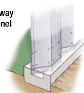
Key-way channel with slab
